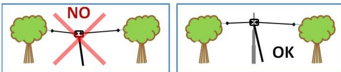
Most people install these antennas as a “Lazy Inverted-V”, with the feedpoint supported by a mast or tree and the ends drooping slightly to remote supports.
